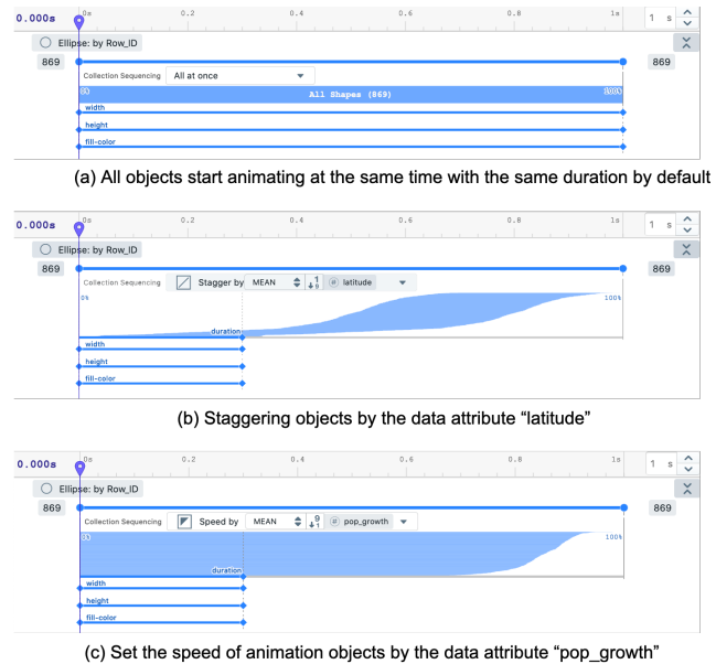
Figure 12: Interface controls for using data attribute values to modify the speed and staggering of animation effects. The middle modification makes the animation start times delay (stagger) as a function of the latitude data attribute. The bottom modification changes the speed to be a function of population growth.
