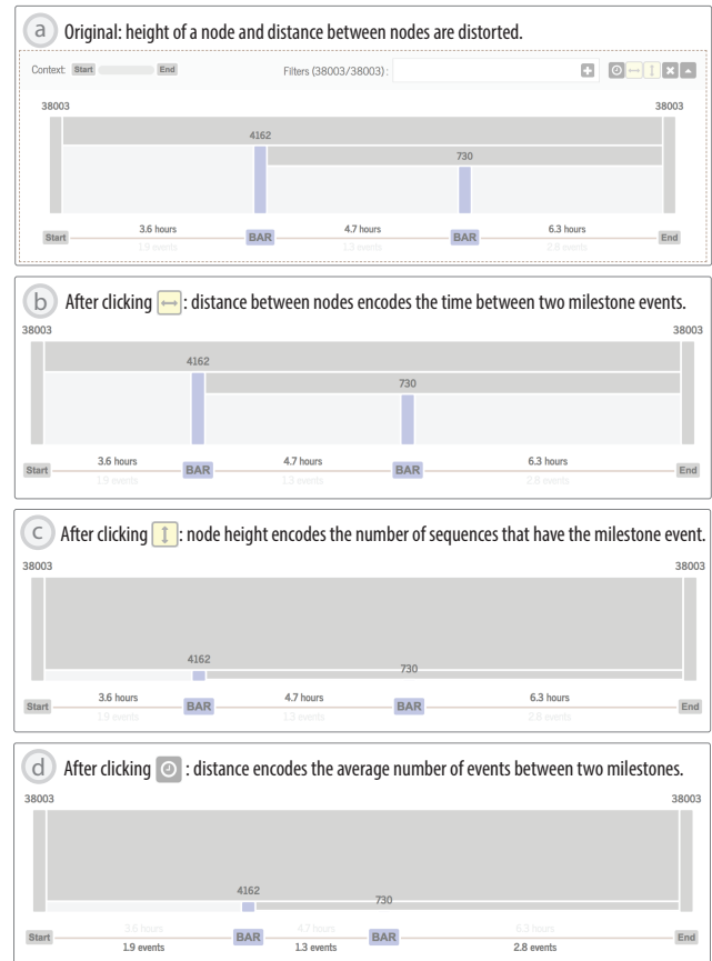
Fig. 6. (a) Node height and horizontal distance between nodes are originally distorted. Analysts can encode distance between nodes as (b) average duration or (d) average number of events in between. They can also encode node height as (c) the number of sequences that contain the milestone event (the number above a node).
